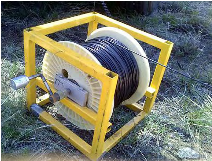
Figure A1. Hand logging winch. Height and length of winch are approximately 18 inches. Width (without winding handle) is approximately 15 inches. Cable has four conductors with an outside diameter of approximately 0.1 inches. Electrical connection while winding is maintained through slip-rings in the far side of the
