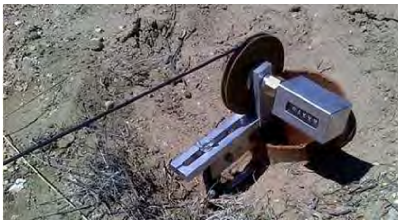
Figure A1. Hand logging winch. Height and length of winch are approximately 18 inches. Width (without winding handle) is approximately 15 inches. Cable has four conductors with an outside diameter of approximately 0.1 inches. Electrical connection while winding is maintained through slip-rings in the far side of the
