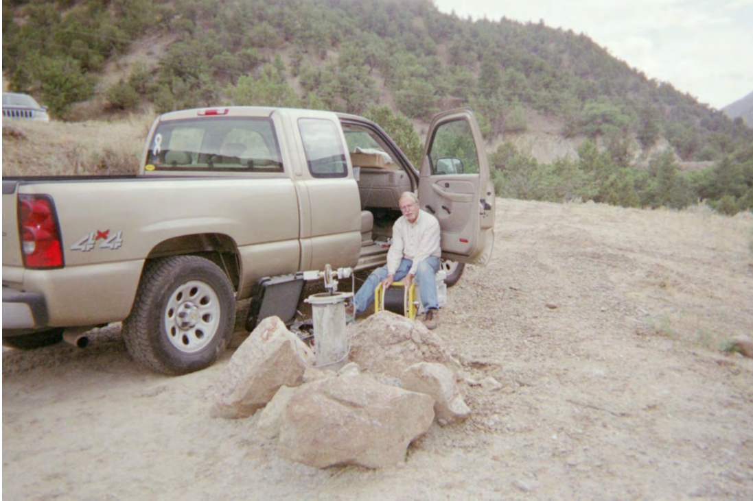
Temperature logging PS-2c at four feet per minute.
